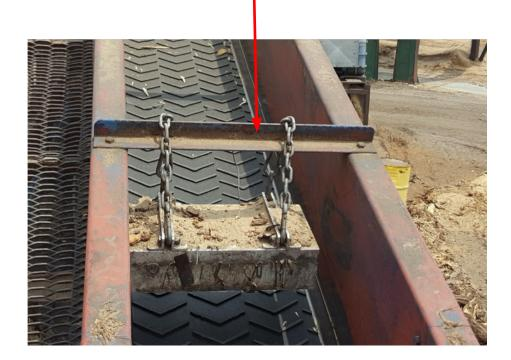
Example of Custom Suspension Mounting Bracket in a Stationary Application.
