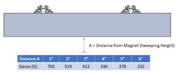
Note: Gauss (G) shown as the peak gauss measured in the center of the magnet at each distance.
