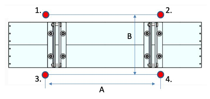
Optimal Dimensions between Suspension Mounting Points
