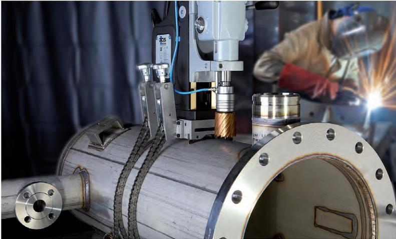
Ideal for applications requiring the flexibility of clamping on pipes from 3-1/4" to 20" diameter. These pipe clamp systems are flexible and easy to use. Swivelling V-blocks fit the contour of the pipe while the heavy-duty tension chains securely affix the clamps to the piece being drilled. The drilling position can be easily and safely adjusted.
