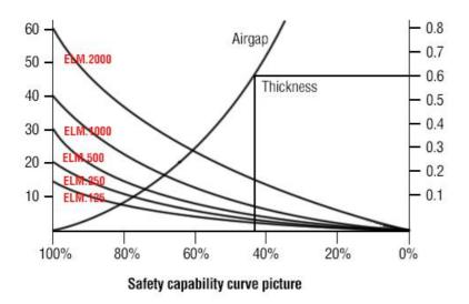
First you calculate the surface roughness (Ra). If this is less than 6.3 um there will be no lifting surface gap and you will have 100% lifting capacity.
