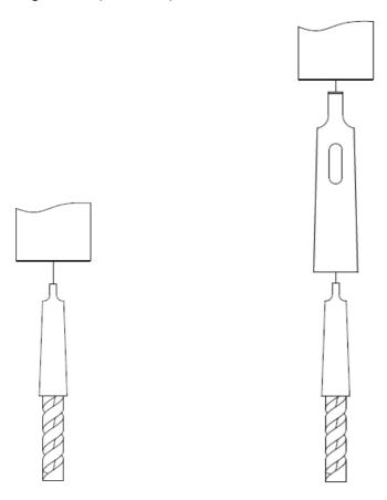
[image 5.3 | fitting drill with MT3 shank] [image 5.4 | fitting drill with MT3-MT2 adapter]
