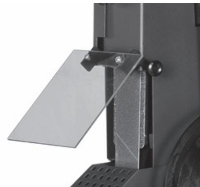
**Figure 4. Eye-shield assembled**
